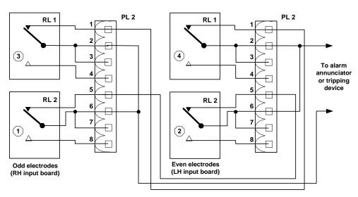
Case B - Relays normally energised, de-energise one pair to trip (Relays shown in de-energised state)
